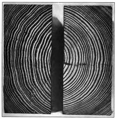
Fig. 25.—Cross section of loblolly-pine beams. Note different proportions of summerwood.
